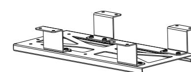
2 Measure and mark the spots to be drilled on (55mm from table edge)
